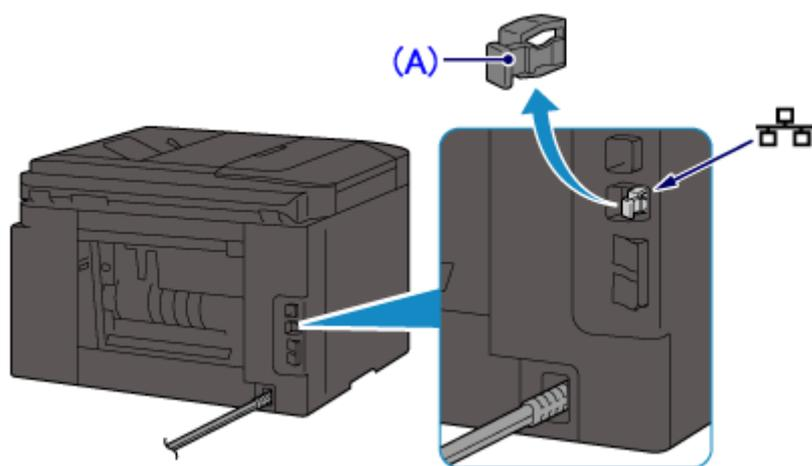
3. Connect the printer and a network device (router, etc.) with an Ethernet cable (B).
