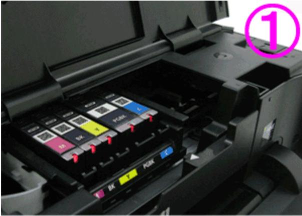
Push the tab (B) and lift the ink tank to remove.
