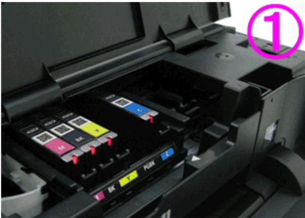
(1) Insert the front end of the ink tank into the print head at a slant.
