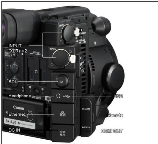
The C200 supports a variety of output signals via HD-SDI and HDMI. High quality on-board audio is delivered via 2 x XLR terminals.
