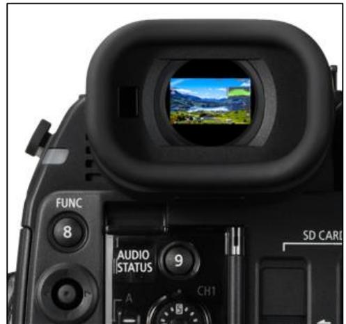
An EVF LUT with partial HDR simulation enables a view close to an HDR display. HDR View Assist (400%/1600%) checking is also possible on the LM-V1.
