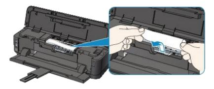
5. Pull the paper slowly not to tear it, then pull the paper out diagonally forward in front at aslant.
